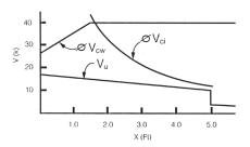
Beyond 5',  $\varnothing V_{ci}$  is the minimum per code while  $V_u$  drops drastically and therefore need not be checked for this case.
